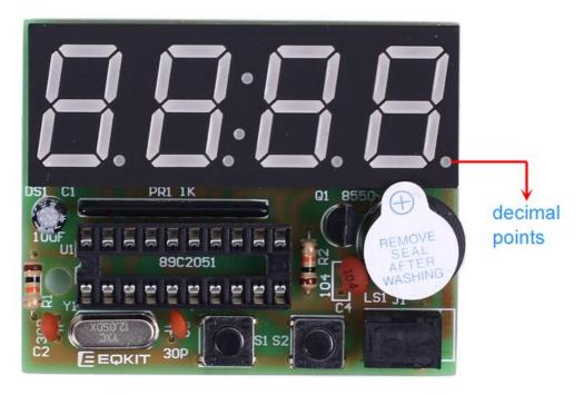
Step 8: Install 1pcs DIP-20 AT89C2051 on IC Socket and pay attention to its installation direction. The AT89C2051 and IC Socket notches are installed in the same direction.
